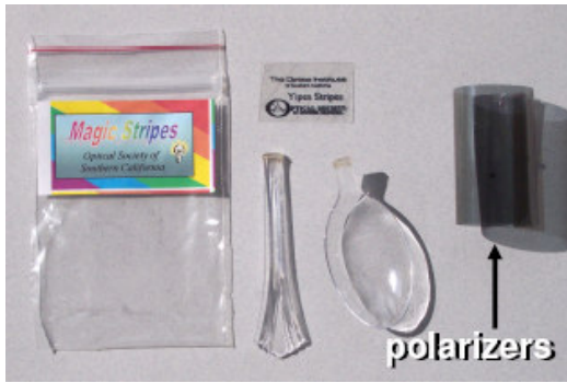
FIG. 4. Equipment for the photoelasticity demonstration.
