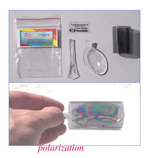
The diameter of the cylindrical Polarizer must be large enough to accommodate the spoon as shown in the photo on the bottom left.
