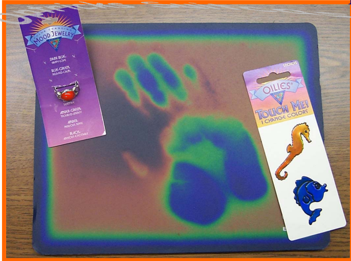
Liquid crystals sense temperature with color
