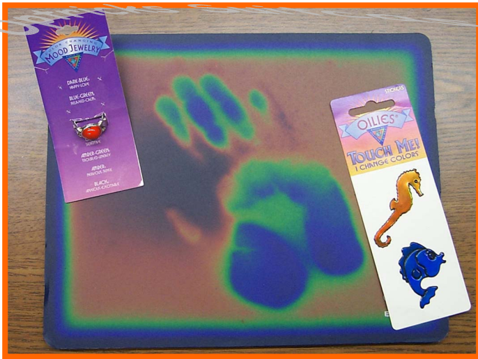
Liquid crystals sense temperature with color
